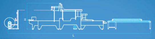
CLM-18000 is an Automatic Carton Lining Machine with advanced features; like Vacuum Belt blank feeding, Web Aligner and Servo Liner Unwind with tension control
